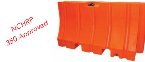
42" x 72" Barricade (Longitudinal Channeling Device) Dimensions: 42"H x 72"L x 24"W Weight: 100 lbs. (.25" / 6.35 mm avg. wall thickness) 130 lbs. (.36" / 9.14 mm avg. wall thickness) 170 lbs. (.44" / 11.18 mm avg. wall thickness)
