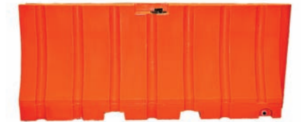
42" x 96" Barricade Dimensions: 42"H x 96"L x 24"W Weight: 150 lbs. (.25" / 6.35 mm avg. wall thickness) 175 lbs. (.36" / 9.14 mm avg. wall thickness) 200 lbs. (.40" / 10.16 mm avg. wall thickness) 250 lbs. (.44" / 11.18 mm avg. wall thickness)
